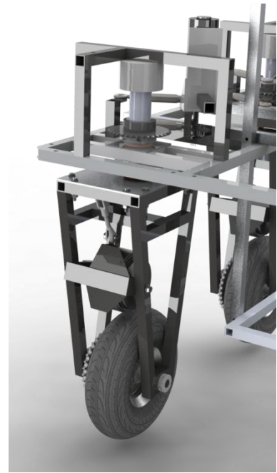
Figure 4.1 One of four drivetrain pods attached to Singularity's frame.
